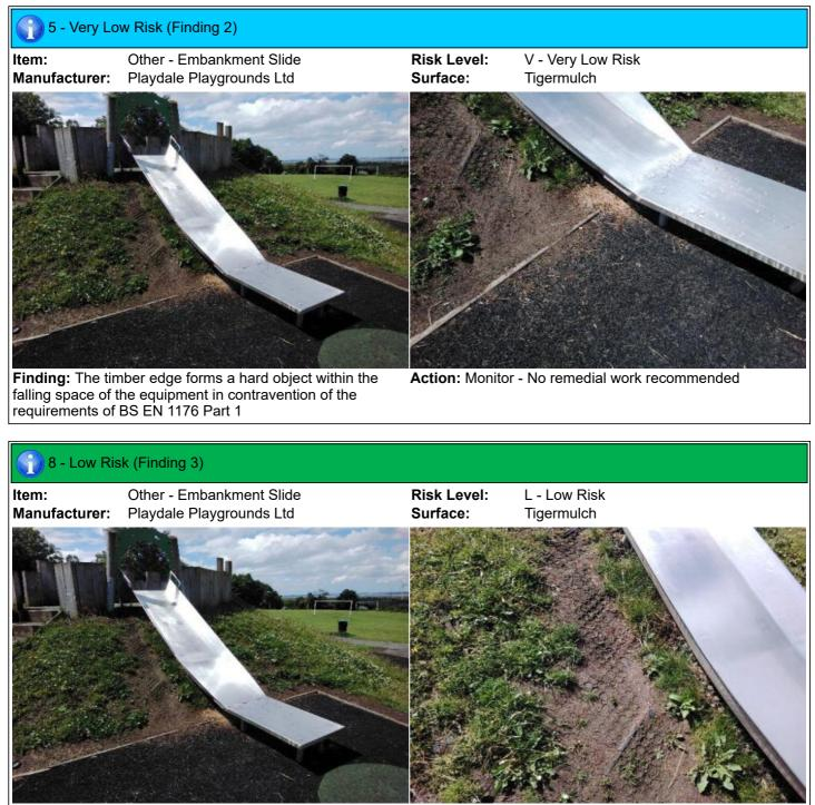
**Finding:** The grass mats are silted up, the soil is compacted **Action:** Reinstate as required and the area will become very slippery when the soil is wet.
