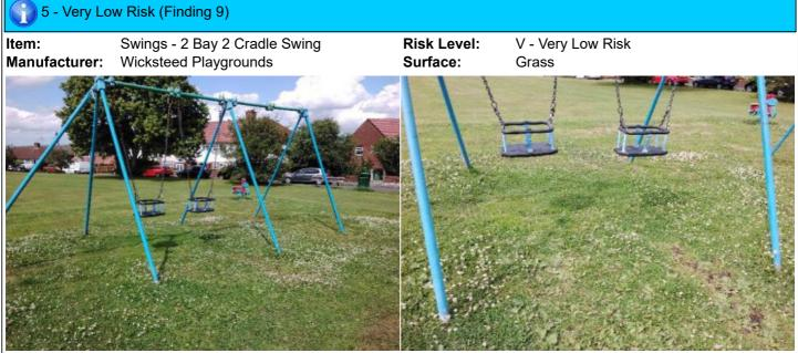
**Finding:** The item of equipment has a fall height exceeding **Action:** Monitor - no remedial action recommended 1.50 metres and grass has been provided as a safety surface
