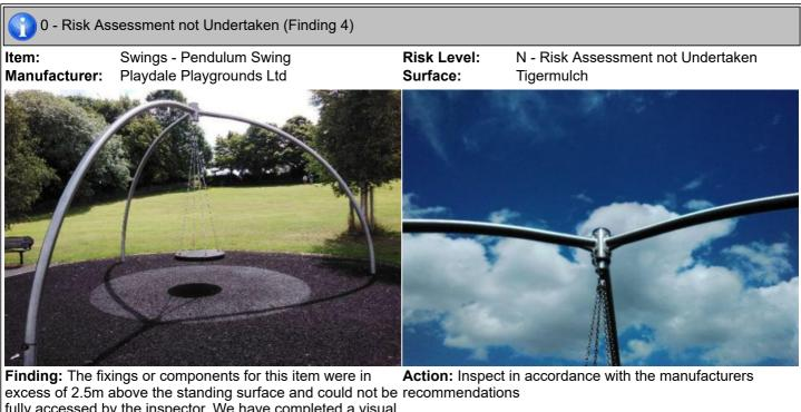
excess of 2.5m above the standing surface and could not be re fully accessed by the inspector. We have completed a visual inspection of the fixings from ground level but a maintenance inspection should be undertaken to assess the condition, security and wear of the components at intervals in accordance with the manufacturers recommendations.
