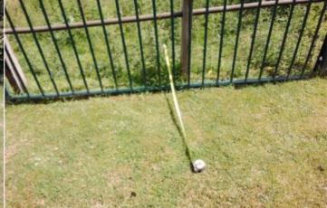
**Finding:** BS EN 1176 requires an additional 1.5m of unobstructed space at each end of the swing surfacing area. This is a relatively low risk finding and no remedial action is recommended at this point.
