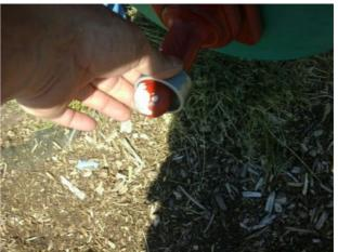
Finding: The end of handgrips and/or footrests have a cross section of less than 15cm2 and fail to meet the requirements of BS EN 1176 Part 6
