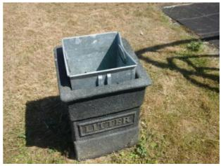
**Finding:** The liner of the litter bin is not secured **Action:** Ensure the lid/door is kept locked and the liner secured
