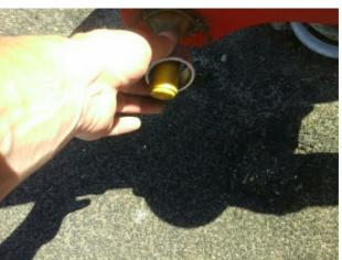
Finding: The end of handgrips and/or footrests have a cross section of less than 15cm2 and fail to meet the requirements of BS EN 1176 Part 6
