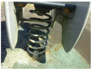
The paintwork on the spring has been damaged or worn exposing the metal underneath which is rusting Finding:
